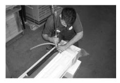
Hold the 90 degree bend root, bend one tube one time. slowly, no quicker than 10 seconds/ 90 degree bend.
