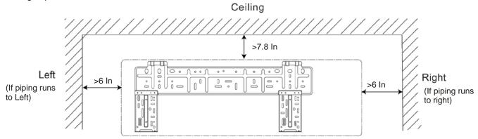
Attention: If there are some additional function devices to install on the unit, be sure add to the installation space for the function devices.
