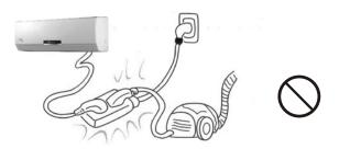
**DO NOT** pull on the power cord or refrigeration lines. Install them in a secured position. A line set PVC cover is recommended.
